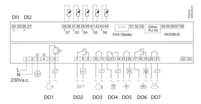
In application 1, the compressors are controlled sequentially. Compressor 1 is first in and last out. In application 3, the compressors are controlled cyclically.
