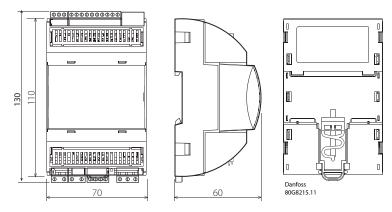
For DIN rail mounting only (IP20)
