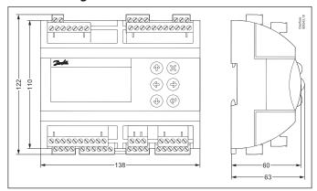
For DIN rail mounting only (IP 20)
